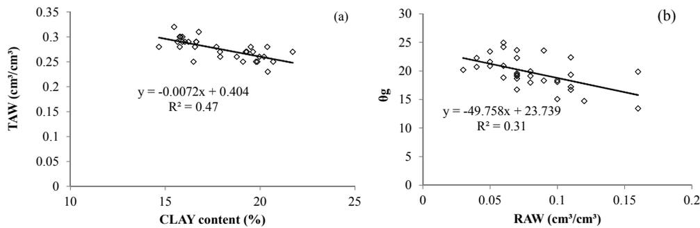
Figure 2. Relationship between TAW (total available water) content and clay content (a) and relationship between average gravimetric water content ( $\theta_g$ ) in 2013 and readily available water (RAW) content (b).
